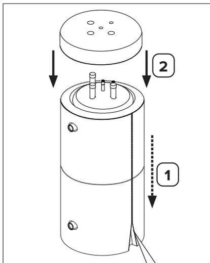
HRs 1000 : Before installing the soft insulation on the tank, assemble the two pieces (zipper).
