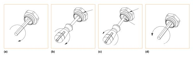
Fig. 1: Lockshield adjustment.
